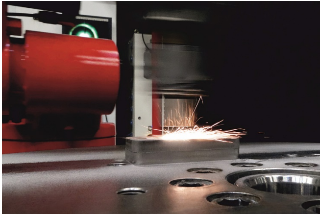
Image 4: In extreme high-speed laser material deposition (EHLA), a new system has made the step from coating to genuine additive, three-dimensional production possible. © Fraunhofer ILT, Aachen, Germany.
